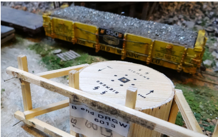
(Above) You can see the label for the cable load as well as the pins which are inserted into predrilled holes in this special flat car.
