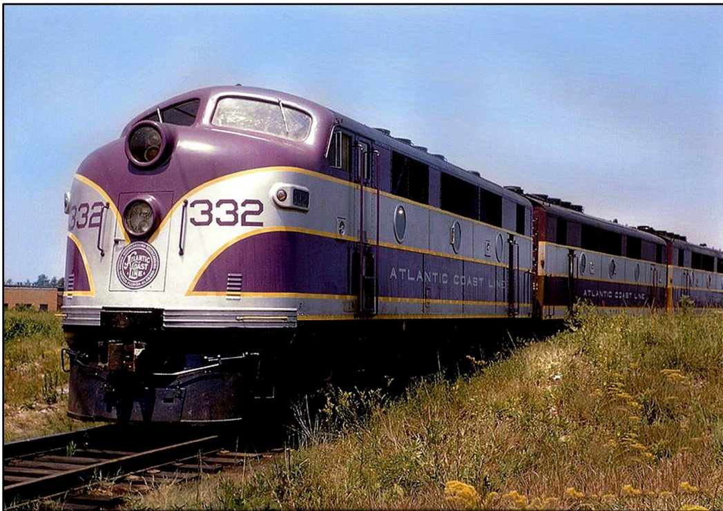
Second Headlight, Small Number boards, Three Portholes, No Chicken Wire, High Fans, all features of the no rhyme nor reason of EMD F2s, but pretty!
