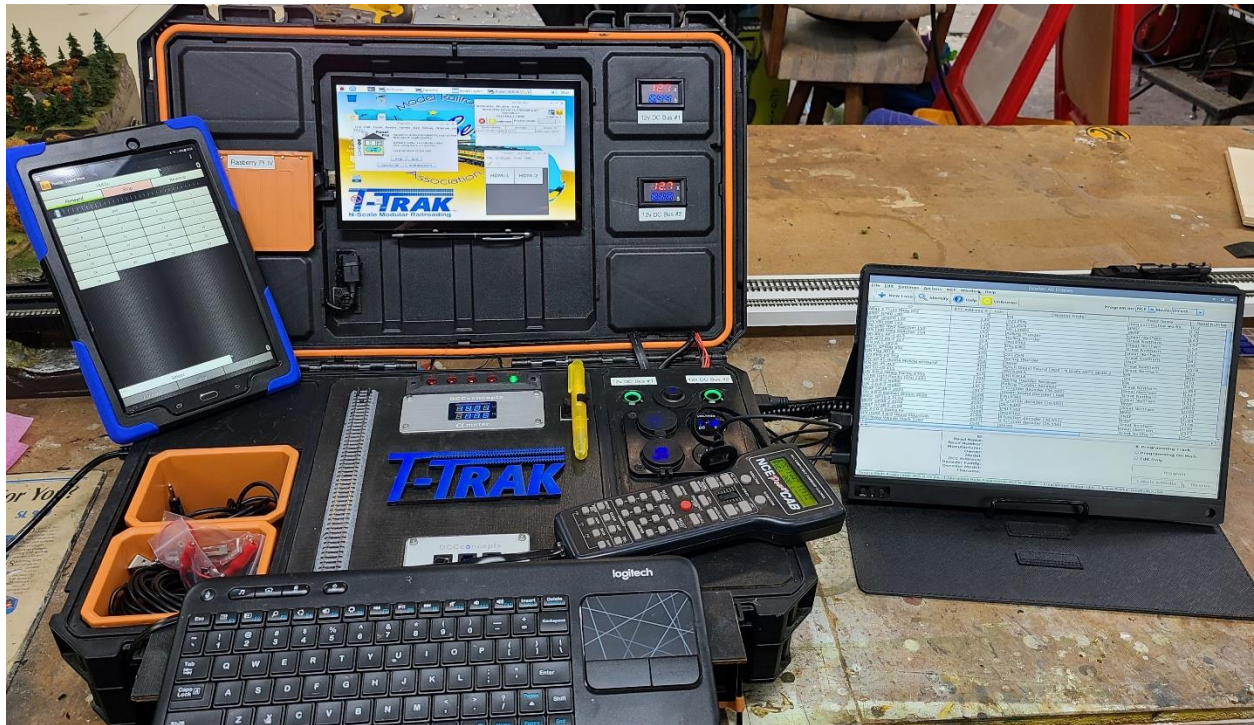
Completed NCE AIO DCC Control System with the secondary monitor
