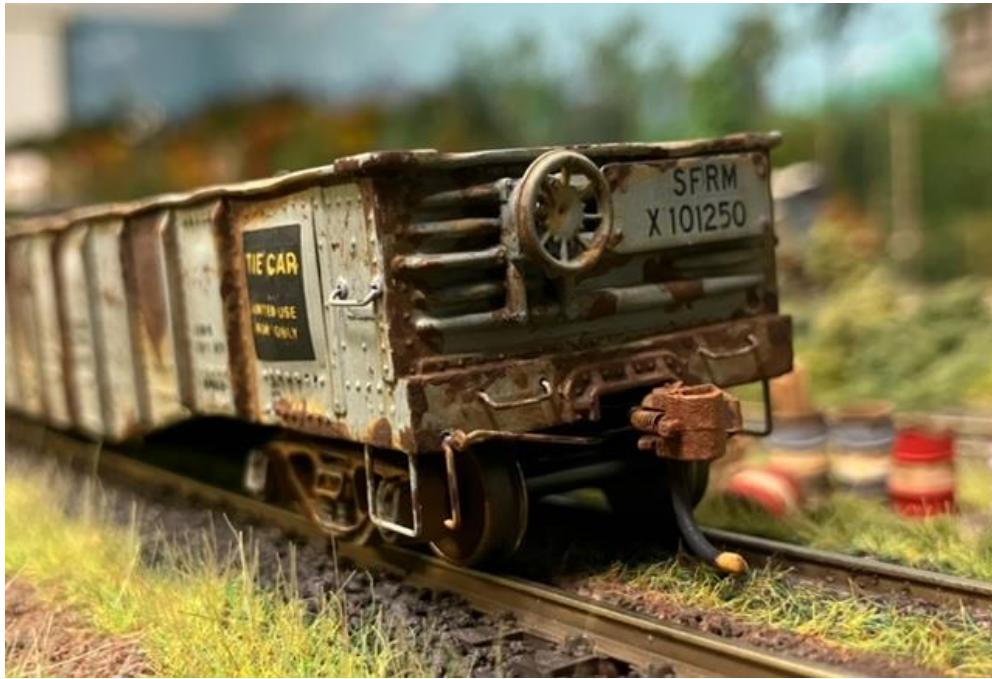
The "B" end of the car details the cut lever, grab irons, deformed upper sill, and reinforced letter panel.
