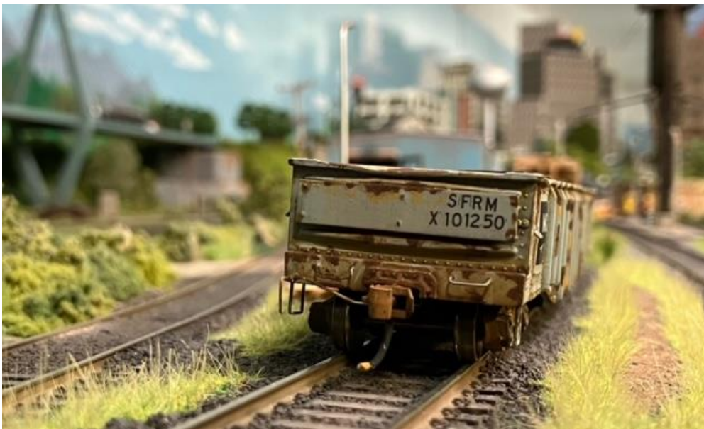
The "A" end with cut lever, grab irons, deformed upper sill, and full width reinforced letter panel.
